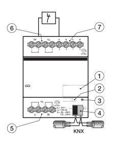
Connecting a 4-conductor sensor with its own power supply
