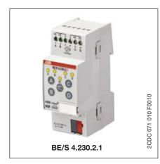
The 4-fold Binary Input BE/S 4.230.2.1 with manual operation is a modular installation device for installation in distribution boards. The device is suitable for detection of 10...230 V AC/DC signals. Inputs A and B are independent of the inputs C and D.
