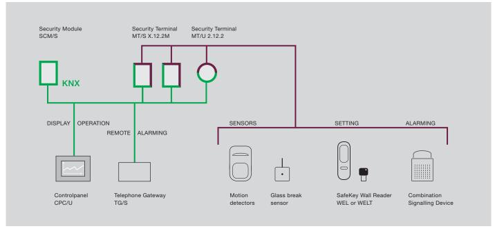
Example of an expansion using Security Module SCM/S
