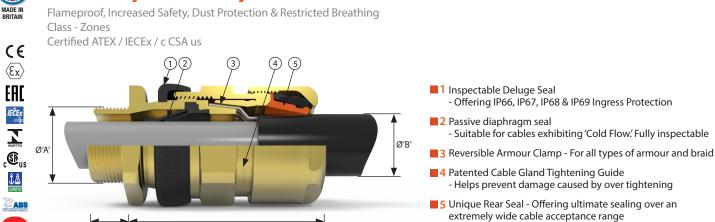
The 501/453 Universal Cable Gland is dual certified Exe/Exd, robust and for use with single wire armour 'W', wire braid 'X', steel tape armour 'Z', elastomer and plastic insulated cables. For particular use with cables that exhibit 'Cold Flow' characteristics. This cable gland is the first and only cable gland capable of being upgraded to a barrier type solution in the field. see below for more details. See technical section for installation rules and regulations.
