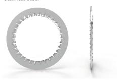
High quality metallic serrated washers designed to designed to protect against loosening of cable gland or locknut in vibrating applications. Often used when mounting a cable gland mounted to a thin wall enclosure, fitted internally with a locknut.
