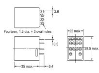
Terminal Arrangement/ Internal Connection Diagram (Bottom View) MY4(Z)H
