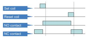
NO contact turns on when voltage is applied to the set coil and stays on even if voltage stops being applied to the set coil. NO contact turns off when voltage is applied to the reset coil, after which NC contact will turn on.\*
