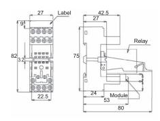
Terminal arrangement/ Internal connections/ mounting holes
