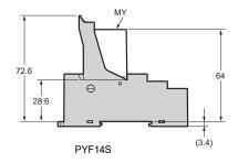
Screw terminal (PYFZ-□(-E), PYF11A, PYF14T, PYF□A-N, PYF14-ES□-B)
