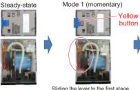
Sliding the lever to the first stage and pressing the yellow button using an insulated flat-blade screwdriver, etc., will operate the contacts
