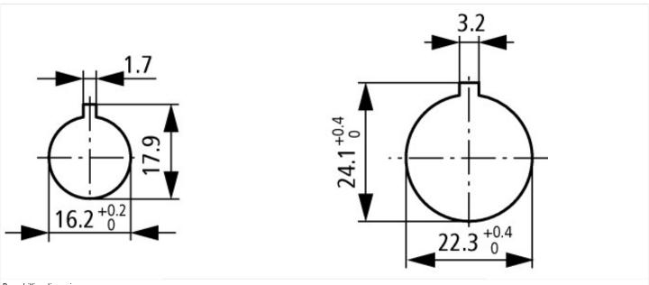
Door drilling dimensions Drilling dimensions: either 16.2 mm = without reduction  $\triangle$  RMQ16 or 22.3 mm = with reduction  $\triangle$  RMQ Titan
