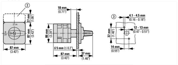
② ZFS-... Label mount not included as standard ③ Drilling dimensions door Cam switches T5B and T5 are same size, only their contacts are different
