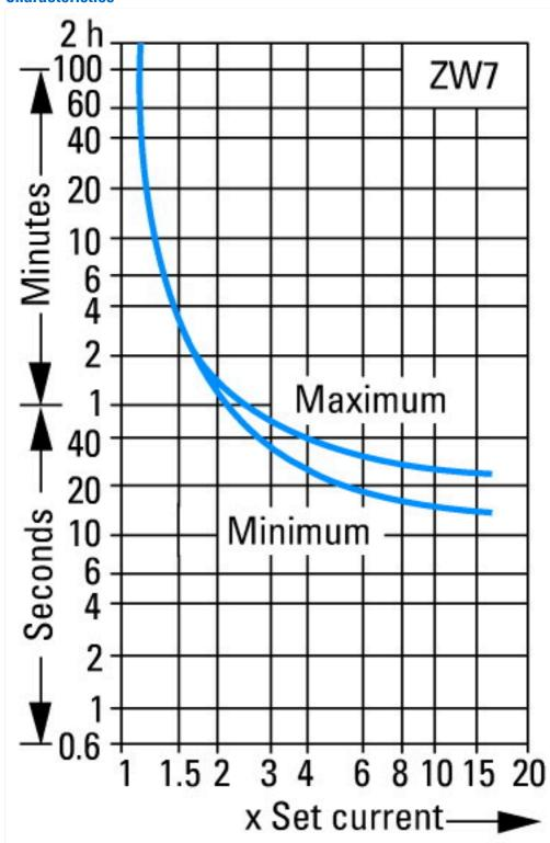
These tripping characteristics are mean values of the spread at 20 °C ambient air temperature in a cold state. Tripping time depends on response current. When the devices are at operational temperature the tripping time of the overload relay reduces to approx. 25 % of the read off value.
