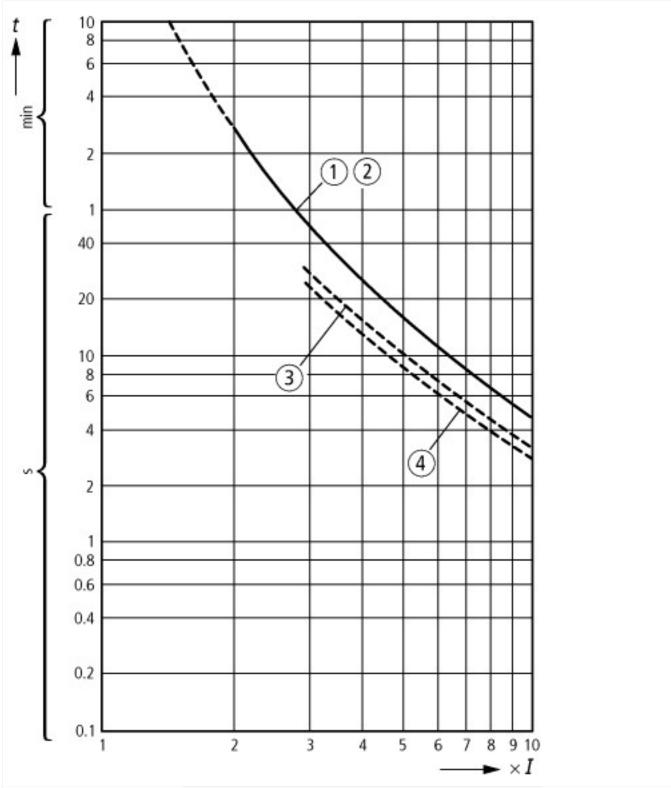
These tripping characteristics are mean values of the spread at 20 °C ambient temperature in a cold state. Tripping time depends on response current.
