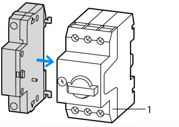
1: Motor-protective circuit-breakers
