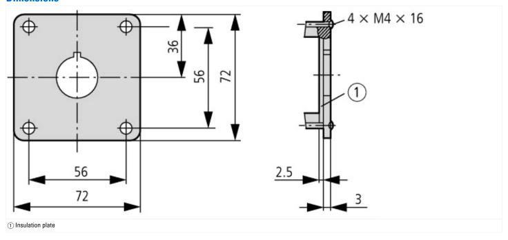
Front fixing (style: flush mounting)
