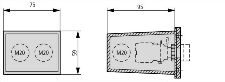
Cable gland: 4 x M20 Construction type: one-piece
