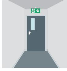
In mains operation, **uniform illumination** of the pictograms facilitates the identification of emergency exits.
