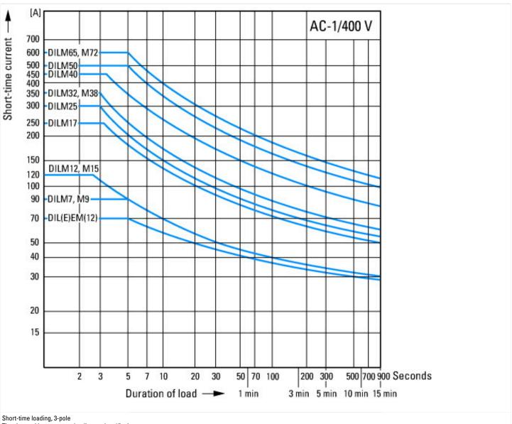
Time interval between two loading cycles: 15 minutes
