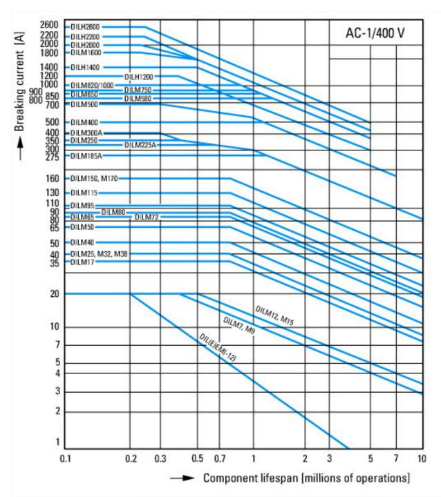
Switching duty for non-motor loads, 3-pole, 4-pole Operating characteristics
