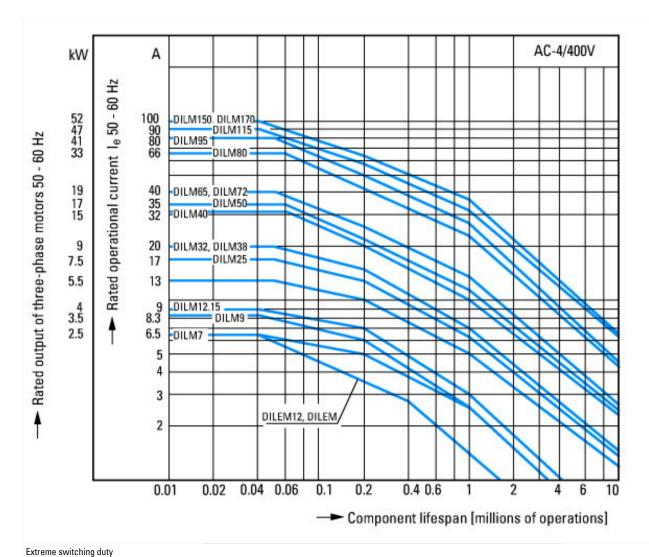
Squirrel-cage motor Operating characteristics Inching, plugging, reversing Electrical characteristics Make: up to 6 x rated motor current Break: up to 6 x rated motor current Utilization category 100 % AC-4 Typical applications Printing presses Wire-drawing machines Centrifuges
