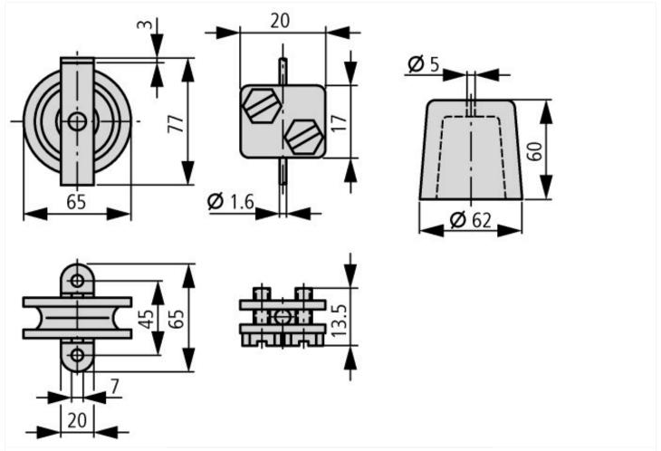
Cable operation: Left: guide pulley Centre: cable clamp Right: 0.9 kg counterweight
