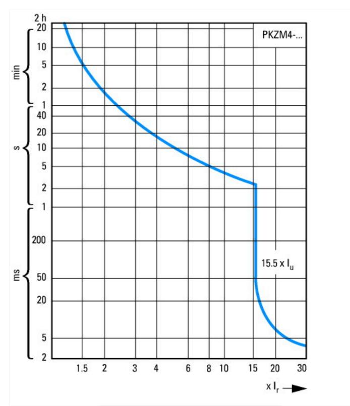
Tripping characteristics motor-protective circuit breaker PKZM4-...
