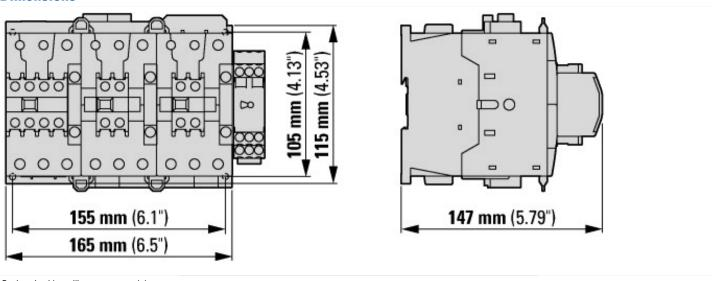
Basic unit with auxiliary contact module
