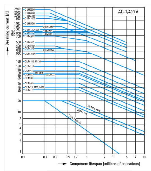
Switching conditions for 3 pole, non-motor loads Operating characteristics
