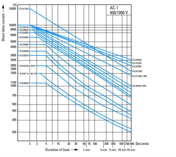
Short-time loading, 3-pole Time interval between two loading cycles: 15 minutes
