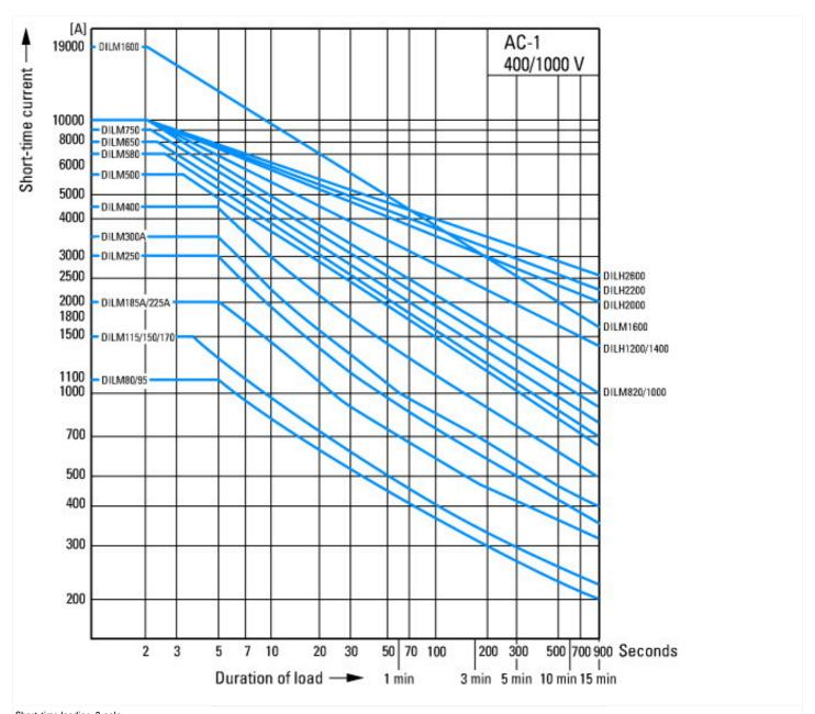
Short-time loading, 3-pole Time interval between two loading cycles: 15 minutes
