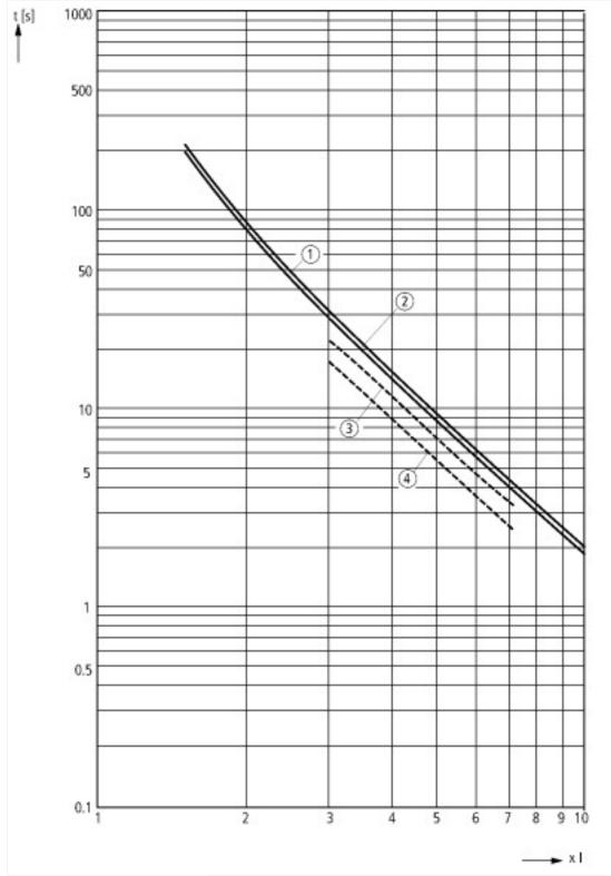
These tripping characteristics are mean values of the spreads at 20 °C ambient air temperature in a cold state. Tripping time depends on response current.
