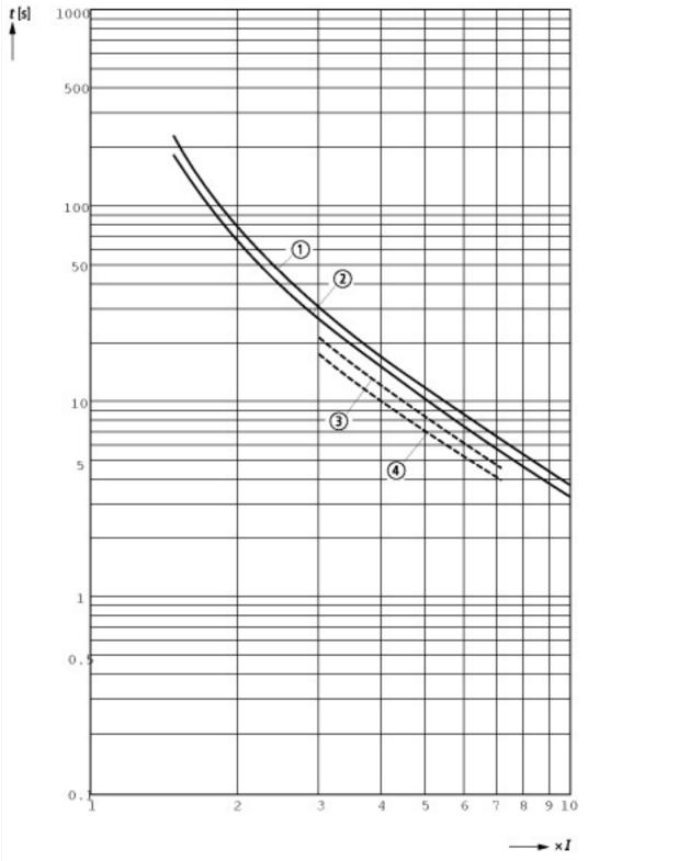
These tripping characteristics are mean values of the spreads at 20 °C ambient air temperature in a cold state. Tripping time depends on response current.
