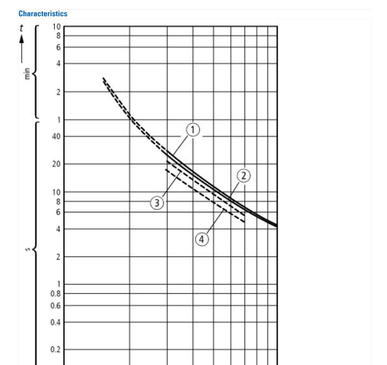
These tripping characteristics are mean values of the spread at 20 °C ambient temperature in a cold state. Tripping time depends on response current.
