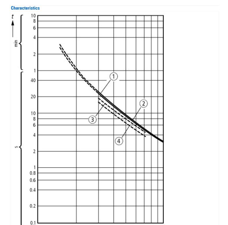
These tripping characteristics are mean values of the spread at 20 °C ambient temperature in a cold state. Tripping time depends on response current.
