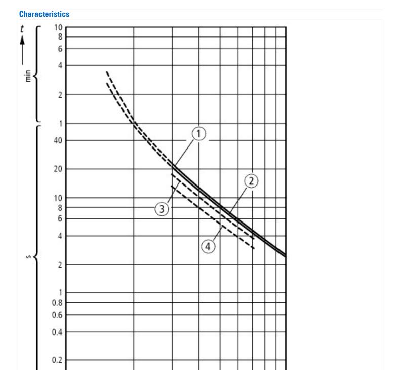
These tripping characteristics are mean values of the spread at 20 °C ambient temperature in a cold state. Tripping time depends on response current.
