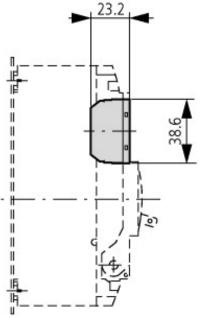
Pushbutton with M22-(C)K... Pushbutton with M22-(C) LED... + M22-XLED...
