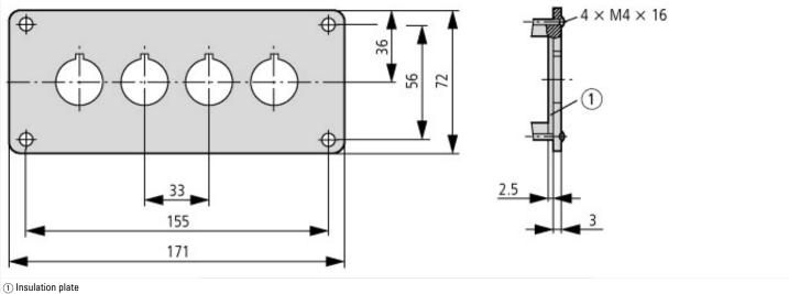
Front fixing (style: flush mounting)
