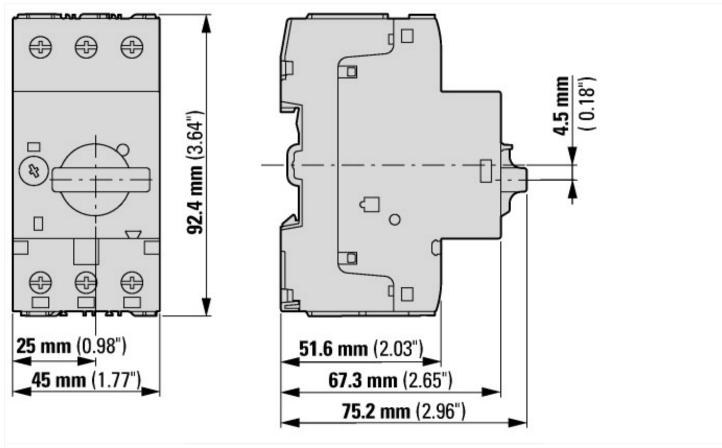
Motor-protective circuit-breaker with standard auxiliary contact
