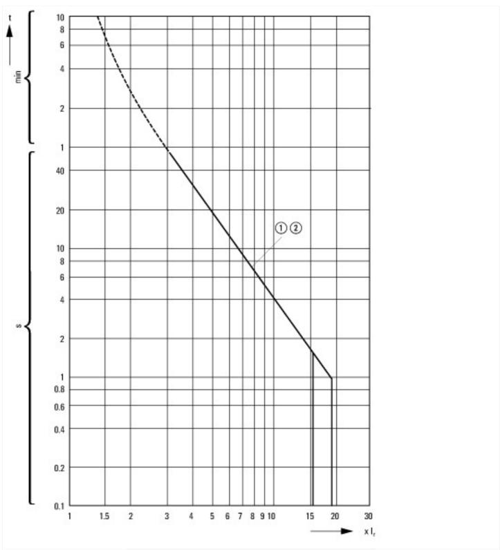
Tripping characteristics motor circuit breaker PKZM0-..., PKZM01
