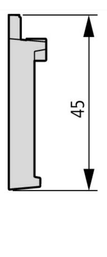
mounting clamp Fixing adapter (front mount) for 4
