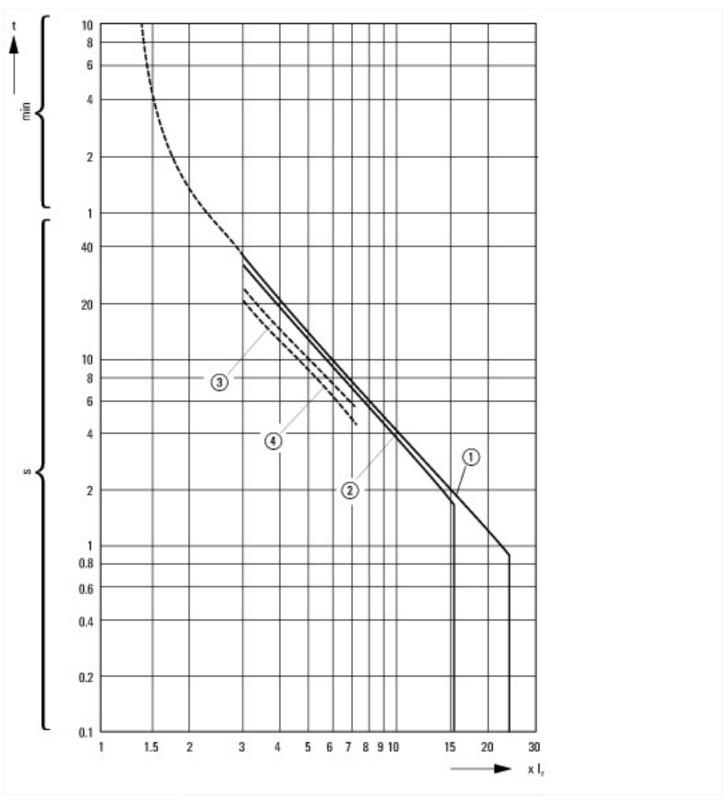
Tripping characteristics motor circuit breaker PKZM0-..., PKZM01
