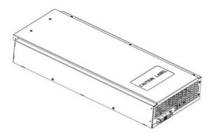
(Figure 10-27: Lithium-ion Battery Module)
