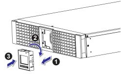
(Figure 6-4: Rotate the Control Panel and the Socomec Logo Nameplate)
