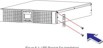
(Figure 6-1: UPS Bracket Ear Installation)
