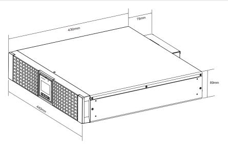
(Figure 2-1: Model 5 / 7 KVA Exterior & Dimensions)
