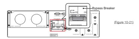
24) Re-install the cover plate of the BYPASS BREAKER on the Manual Bypass. This will automatically inactivate the manual bypass detector.
