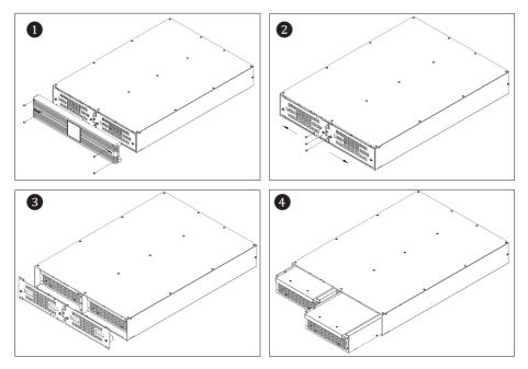
(Figure 10-28: Install the Lithium-ion Battery Module(s))
