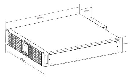
(Figure 2-2: Model 9/ 11 KVA Exterior & Dimensions)
