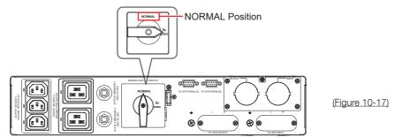
16) Re-install the cover plate of the MANUAL BYPASS SWITCH on the Manual Bypass. This will automatically inactivate the manual bypass detector.
