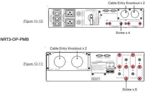
3 Follow *Figure 10-12* and *Figure 10-13* to install the provided accessories on the Manual Bypass and perform wiring. The suggested knockout or hole diameter for optional cable gland is 34.5mm (1-23/ 64 inch).
