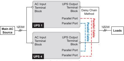
(Figure 7-4: Parallel Units Wiring Diagram)
