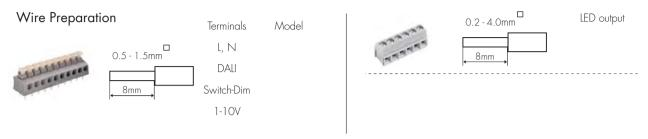
To make or release the wire from the terminal, use a screwdriver to push down the button.
