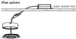
3. Fix the mounting base to the cabinet with screws. Push the luminaire up into mounting base. Ensure that it is securely located.
