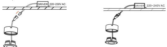
3. Fix the mounting base to the cabinet with screws. Push the luminaire up into mounting base. Ensure that it is securely located.
