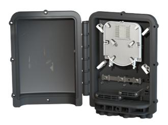
This ruggedised splice enclosure is designed to allow up to 60 individual fibres, incorporating a hinged door to provide easy access for installation and re-work. The enclosure is suitable for a range of harsh environments with an impressive IP68 rating. It can be placed in aerial, wall mounted, or duct mounted locations.
