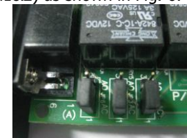
Fig. 6 Jumper setting for ACTIVE CLOSE
