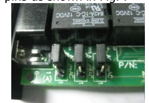
Fig. 7 Jumper setting for ACTIVE OPEN
