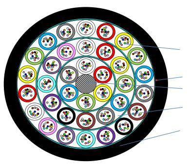
Loose buffer tubes, diam. 2,3mm each with up to 12 fibers, filled with a thixotropic gel,
