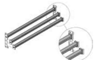
Quick installation, each busbar is lifted into place separately from the front prior to attachment.
