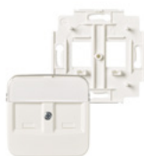
RJ45 outlet with sliding dust covers The RJ45 inserts and center plate are made for 2 connectors. The connectors are not included. The connectors CEL30.UX are not compatible with this device, due to its integrated dust covers.
