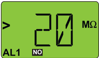
Figure 8:Insulation resistance > 20MΩ.
