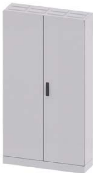
ALPHA 630 DIN FLOOR DISTR.BOARD IP55, SK II, RAL 7035 H=1950 W=1050 D=320 INCL. BASE AND SHEET-STEEL DOOR WITH CLOSED SIDE PANEL
