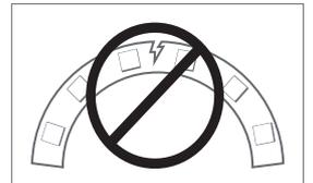
EN: Do not bend LED strip on horizontal plane, do not fold, crease, or twist LED strip.
