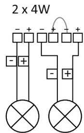
EN: **NB.** When connecting several luminaires to the same dimmer it's important to allocate the same number of luminaires to the drivers (preferably maximum load and rather use more drivers than uneven distribution across fewer drivers). This is to avoid light differences.
