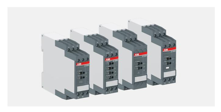
The advanced CT-S range includes 22 single-function devices and 16 multifunction timers with up to 13 functions. The devices feature seven or ten time ranges, which are adjustable from 0.05 seconds to 300 hours. Every device is available in two different connection technologies: double-chamber cage connection terminals or ABB's vibration-resistant Push-in Technology.
