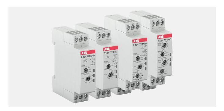
The CT-D range is ideal for building applications and installation panels, due to its compact modular housing. For maximum flexibility in operation, nine single-function as well as two multifunction devices with seven timing functions are available. The devices offer four or seven time ranges from 0.05 seconds up to 100 hours. Their wide supply voltage range allows their use in applications worldwide.
