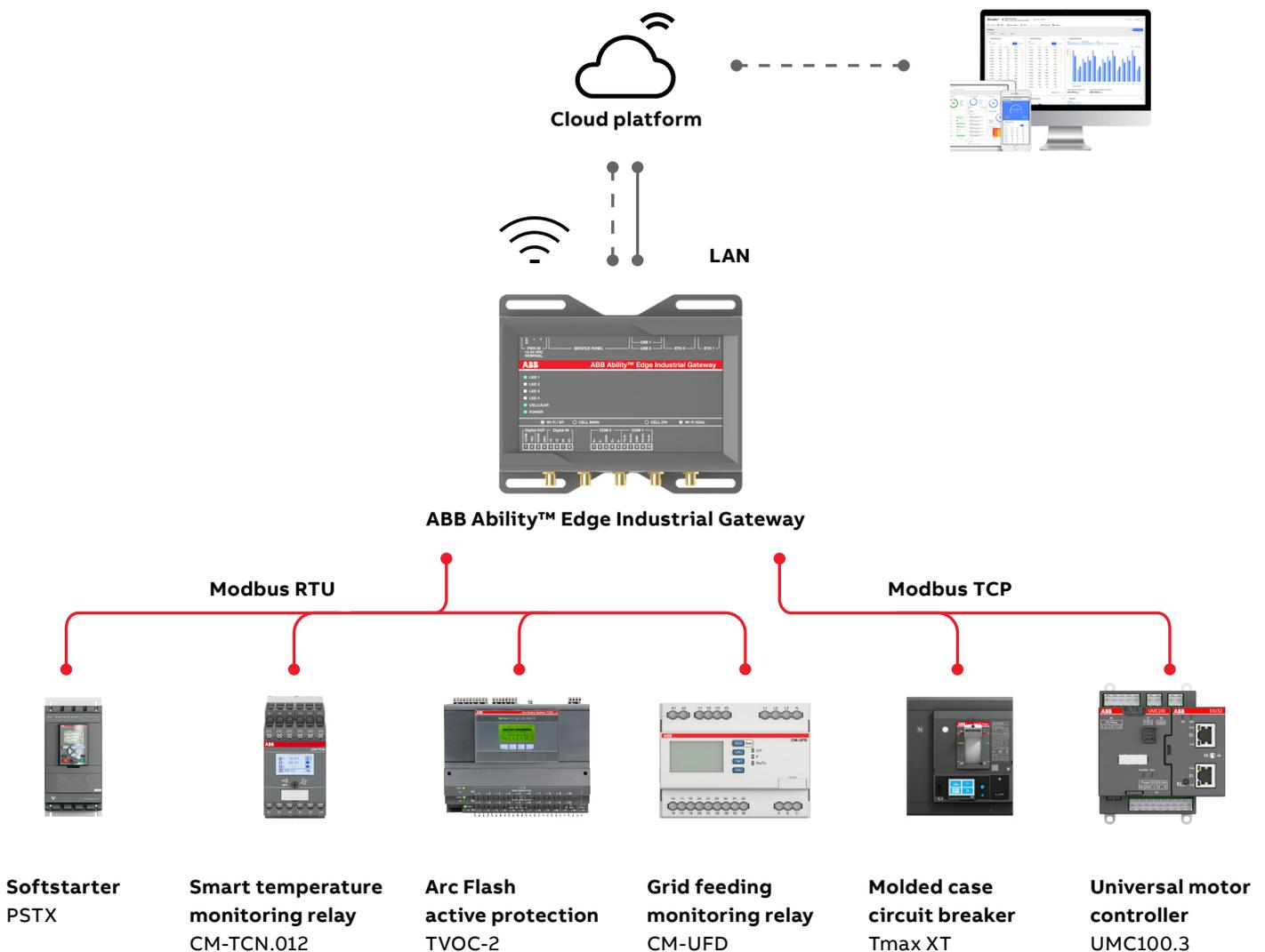
Integrate a range of devices like circuit breakers, motor controllers and the new CM-TCN.012 monitoring relay into the ABB Ability™ Energy Manager and ABB Ability™ Asset Manager. It is a state-of-
