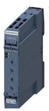
TIME RELAY, ELECTRONIC, FLASH. RELAY ASYMMETRICAL, 1 CO CONT., 15 TIME SET. RANGES 0.05S...100HR, 12...240V AC/DC AT AC 50/60HZ, LED, SPRING-LOADED TERMINAL (PUSHIN)
