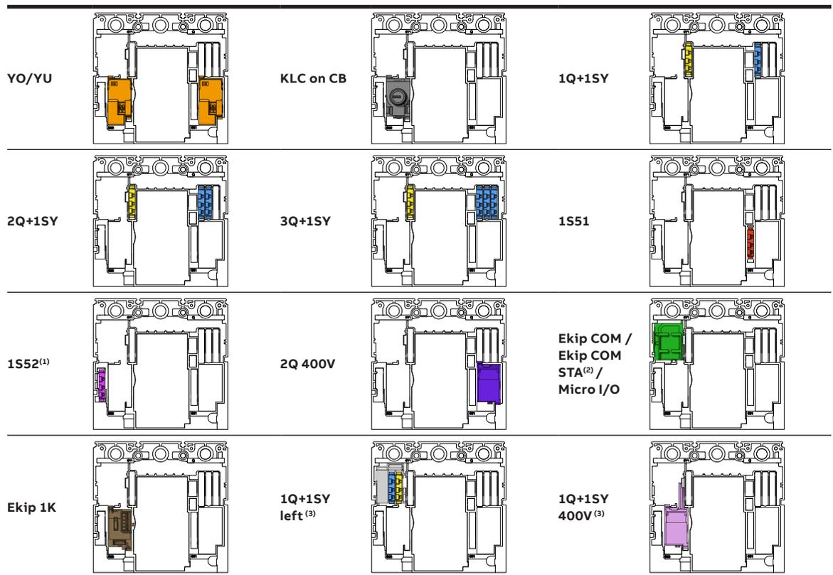
(1) YO or YU must be mounted on the third pole to make S52 signaling available.
