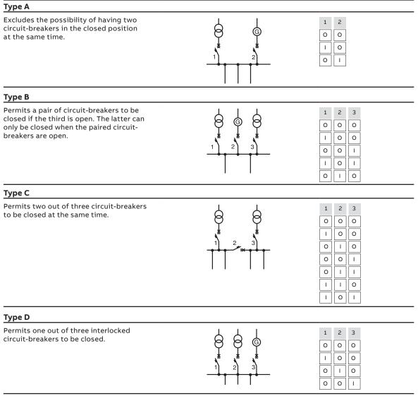
The mechanical interlocks offer multiple solutions for installation that simplify their integration into the switchgear. The interlocks can be mounted:
