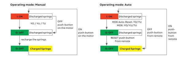
With the XT5 MOE and MOE-E and the XT6 MOE, it is possible to define some reset logic in order to charge the springs automatically once the circuit-breaker has tripped depending on the reset wiring diagram chosen. Three different options are available:
