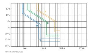
Fig. 2 - Protection thresholds during on-grid operation
