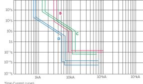
Fig. 3 - Protection thresholds during islanded operation
