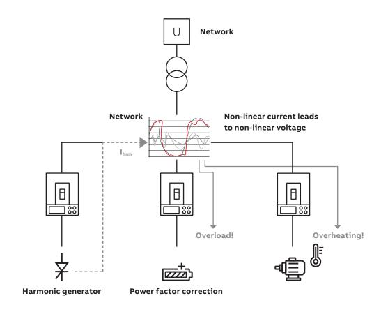
Power electronics produce harmonic content that can affect other loads in the plant: the result can be an overheating of the asynchronous motor and an overload (that could lead to a trip of the protecting MCCB) on the power factor correction capacitors.
